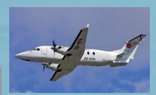
The **BEECHCRAFT 1900-D** is multi crew, has twin engines and is operated under Instrument Flight conditions, enabling flights in bad weather (clouds, rain, etc.).
